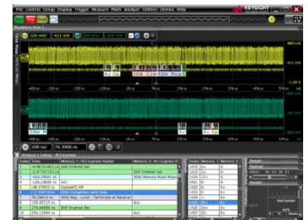
Trigger on and decode PCIe serial packets.
