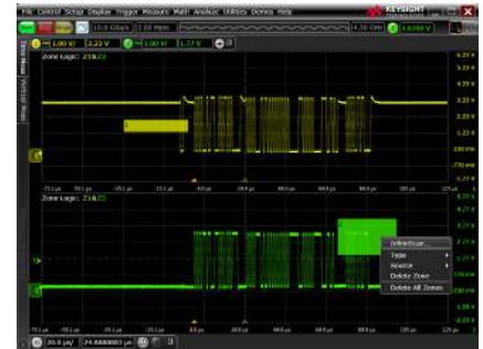
Identify signal integrity issues with IniniiScan Zone – Quality triggering.
