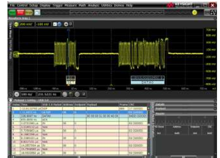
Trigger on and decode USB packets.
